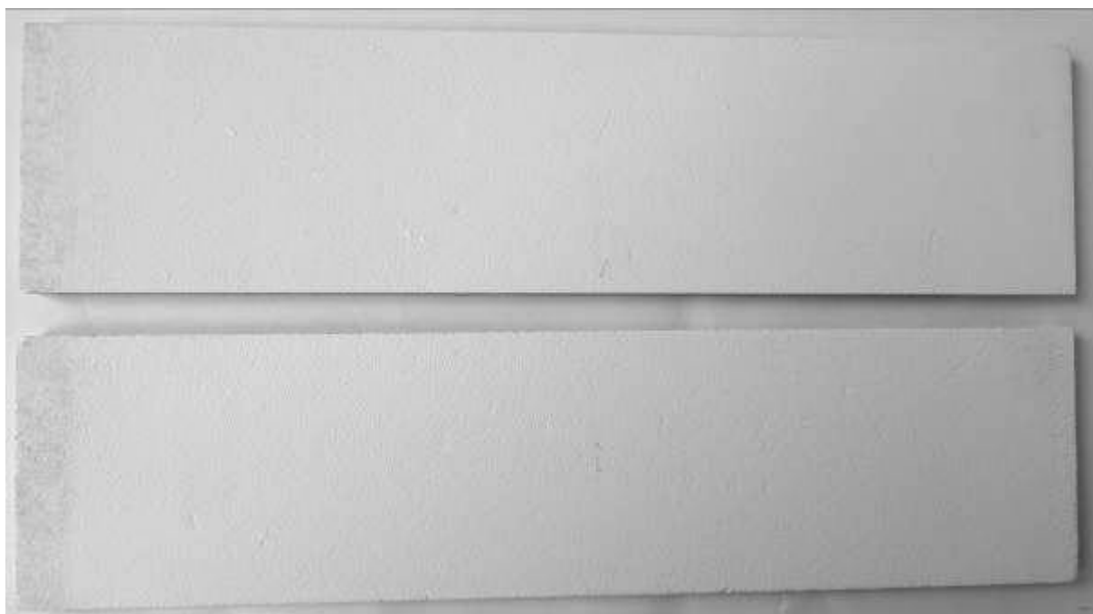
Photo of samples no. 3, 4 Exposure to UV lamps for 1500 hours
