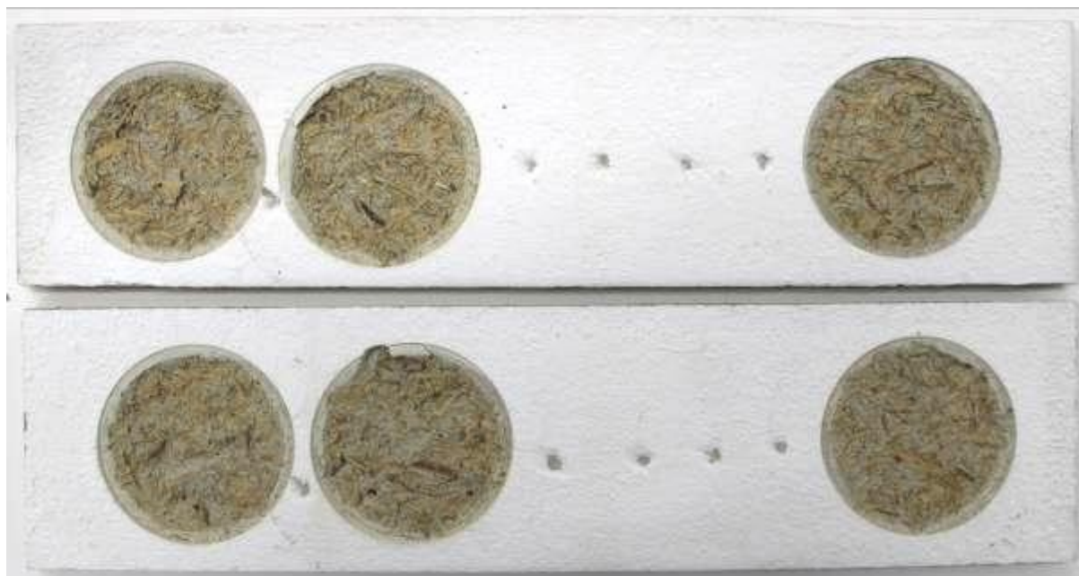
Photo of parts no. 3, 4 after tear test – exposure 2000 h under UV lamps
