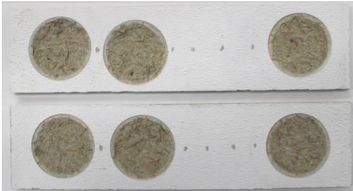
Photo of parts no. 3, 4 after tear test – exposure 2000 h under UV lamps
