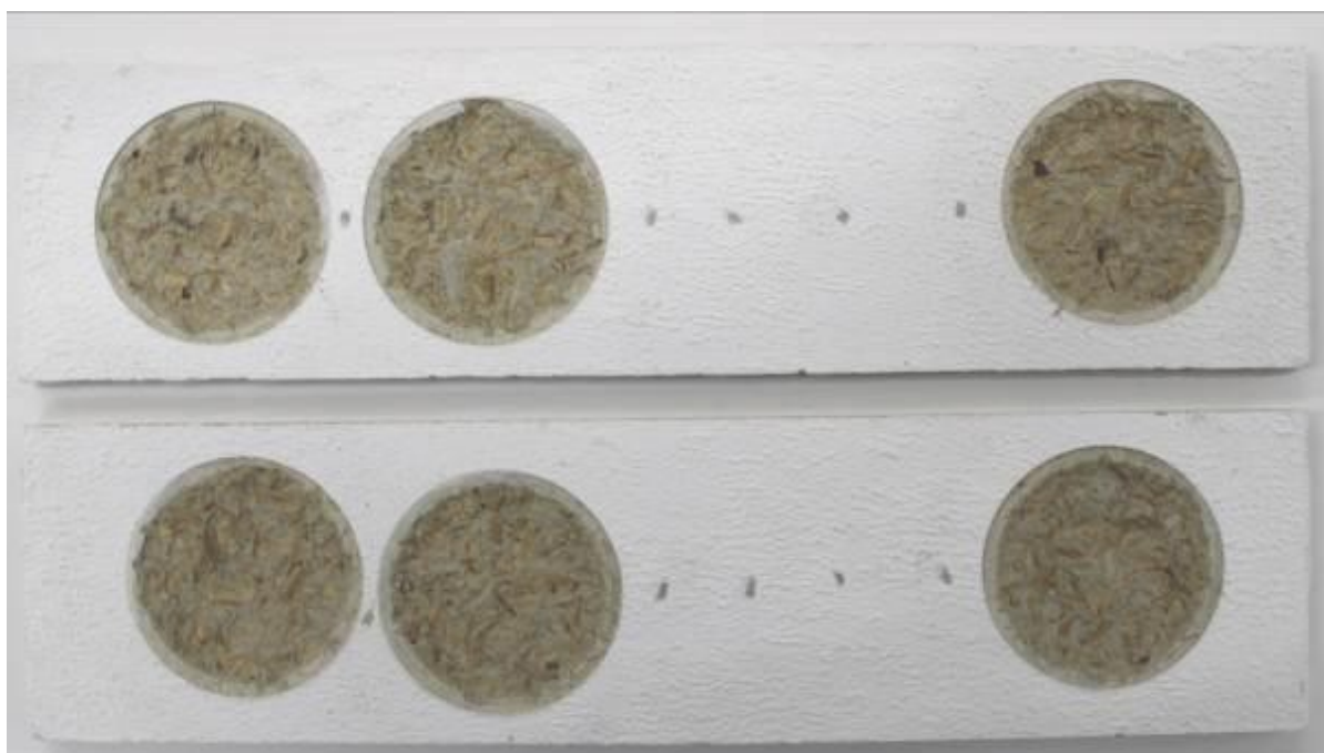
Photo of parts no. 1, 2 after tear test - without exposure
